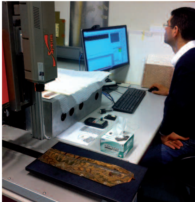
70 A gilt leather fragment from the Rijksmuseum Amsterdam on the scanning platform under a hyperspectral imaging camera.
