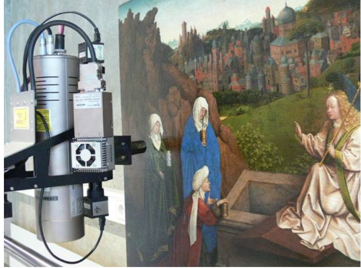
Image 16: The macro-X-ray fluorescence (XRF) scanner scans Jan van Eyck's Three Marias at the grave (c. 1425-1435; panel 71.5 x 90 cm, Museum Boijmans van Beuningen, Rotterdam). The macro-XRF scanner, developed by TUDelft and the University of Antwerp, provides in a non-destructive manner a two-dimensional image of the elemental composition; this gives information about the paint composition, paint layer structure and painting technique (research: TUDelft, NWO).
