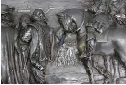
Image 12: Matthias Melin, General Ambrogio Spinola during the siege of Gulik in 1622 , silver 23.5 x 54.5 cm, Rijksmuseum. Severe stress-corrosion cracking in this bas-relief plaque in embossed silver has resulted in a large hole in the middle of the scene. The causes of cracking in embossed silver are still not very well studied. However the effects of this ageing phenomenon are dramatic and lead to loss of material in many more objects than is currently recognized (research J. Van Bennekom, et al.; Rijksmuseum, National Aerospace Laboratory).
