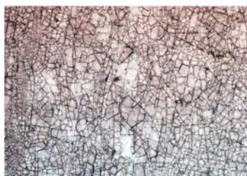
Image 10: This beautifully engraved beaker (England ca. 1676, Corning Museum) is seriously damaged as a result of “glass disease”. There are numerous tiny cracks throughout the glass (see detail from a similar glass), which cause the glass to lose its transparency. “Glass disease” occurs because the earth-alkali ions, which are added during the fabrication process to lower the melting temperature of the glass, slowly leach out of the glass over time. The leaching of the earth alkali ions results in changes in the glass composition and tension within the glass. Primarily with rapid changes in relative humidity, miniscule cracks form in the glass (research: G. Verhaar, N.Tennent, M. van Bommel, B. Lamain UvA/RCE/Rijksmuseum).
