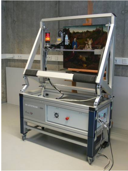
Image 16: The macro-X-ray fluorescence (XRF) scanner scans Jan van Eyck's Three Marias at the grave (c. 1425-1435; panel 71.5 x 90 cm, Museum Boijmans van Beuningen, Rotterdam). The macro-XRF scanner, developed by TUDelft and the University of Antwerp, provides in a non-destructive manner a two-dimensional image of the elemental composition; this gives information about the paint composition, paint layer structure and painting technique (research: TUDelft, NWO).
