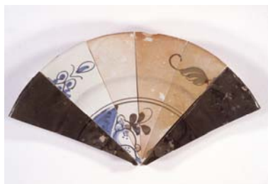
Image 11: After excavation of Delft plate (1670-75) from a cesspit, it was determined that the formerly deep blue and white lead glaze had been converted to a black lead sulfide by micro-organisms. One method to re-convert blackened glazes to their original composition and thus restore the blue and white colors, is to re-fire the plate. The outer left and right sherds, which have not been heated, exhibit the black lead sulfide-containing glaze. The SEM results show crystals of the black lead sulfide from the sherd after burial in a cesspit. The four sherds in the middle show the effect of re-firing in an oxidizing oven; each is re-fired at a single temperature between 560°C and 920°C. At the highest firing temperature, second sherd from the left, enough of the original glaze is re-formed to restore the blue color. The current research focuses on the restoration of the blue-white glaze by means of photochemical conversion of lead sulfide. This method is not only milder than re-firing but also produces better results (research: N. Tennent, UvA).
